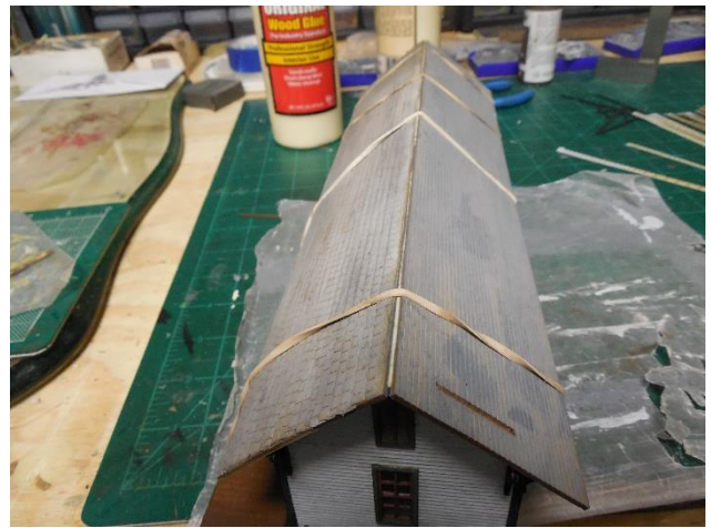
Pic 14: Peel-and-stick shingles have been applied to the roof panels. Rubber bands were used to hold the panels in place while glue dried.
