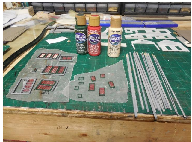
Pic 9: Window castings and trim strips are pre-painted and ready for assembly.
